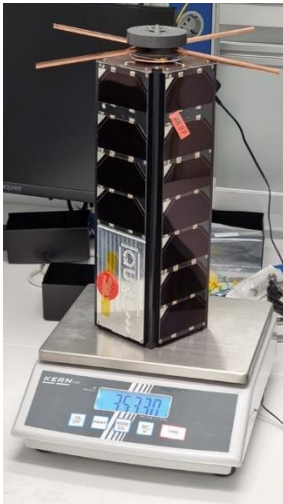
Photo 2: QUBE mass determination (© Zentrum für Telematik) The flight model of the completed QUBE exhibits only a mass 3.533 kg to provide all functionalities for technology tests on quantum key generation and transmission.
