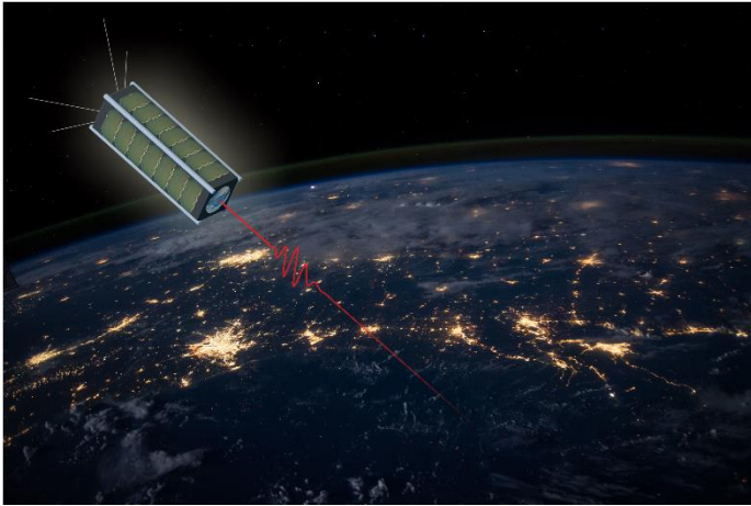
Photo 1: QUBE technologies for quantum key distribution (© Zentrum für Telematik) The objective of the QUBE nano-satellite is to transmit quantum keys with a laser to the ground station, supporting future secure communication on Earth.
